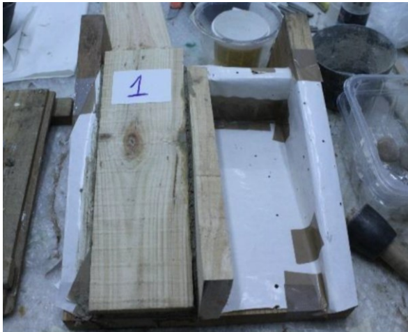
Replicating original formwork
